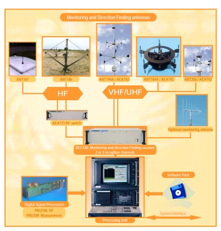
ESMERALDA has also other configurations: independent direction finder (also referenced TRC8000) or monitoring and measurement receiver fitted with 1 up to 4 independent channels (also referenced TRC8025).
